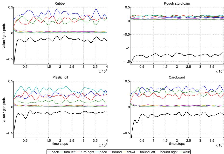
**Fig. 3.** Value (black curve under the abscissa) and gait selection frequencies (above) over time on 4 ground substrates (data from simulator). All curves have been smoothed with a weighted linear least squares and a 2nd degree polynomial model in a moving window of 5.000 samples. To appreciate the time course of the value function, the initially low values have been clipped. Note the different scale of the value function for rough styrofoam.
