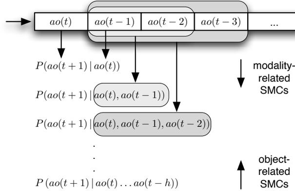
**Fig. 1.** Schema of the proposed computational model of SMCs. The sequence of actions and sensory observation ( $ao$ ) is used to train Markov models of different history lengths  $h$ . We suggest that object-related SMCs are captured by models with longer context sizes, and modality-related SMCs by models with a short context.
