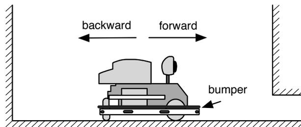
**Fig. 2.** Profile view of the experimental setup. The robot could freely move forward and backward between the two walls. The shape of the front wall (right) stopped the movement, but did not trigger the bumper.
